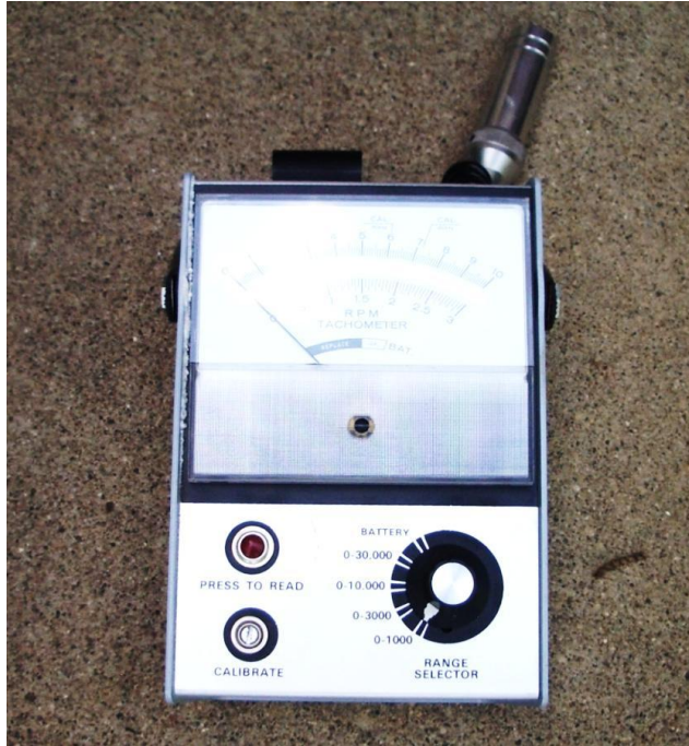
Figure 4.13 – Photo reflective tachometer.
