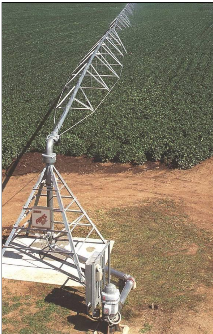
Figure B.2 - Center pivot sprinkler irrigation system.
