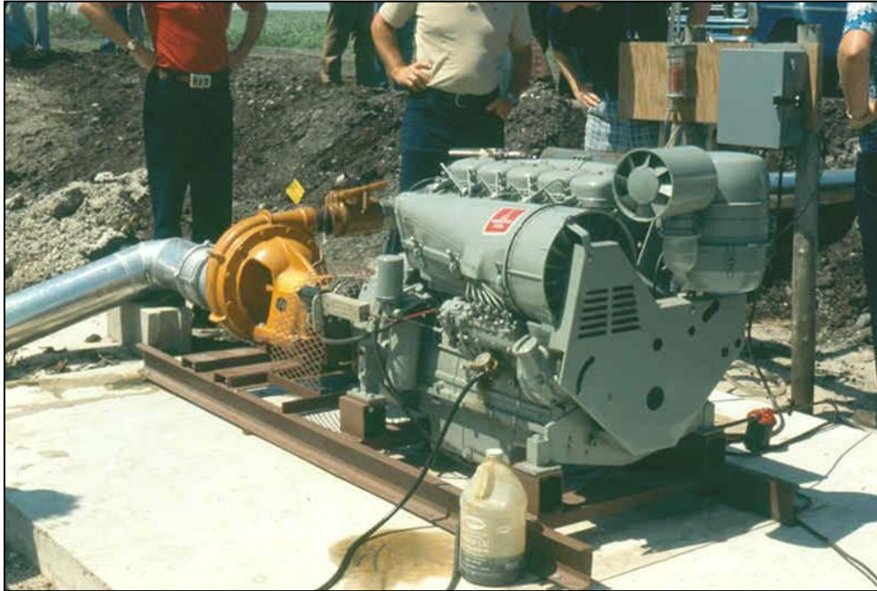
Figure 3.4 - Centrifugal pump with diesel power unit.
