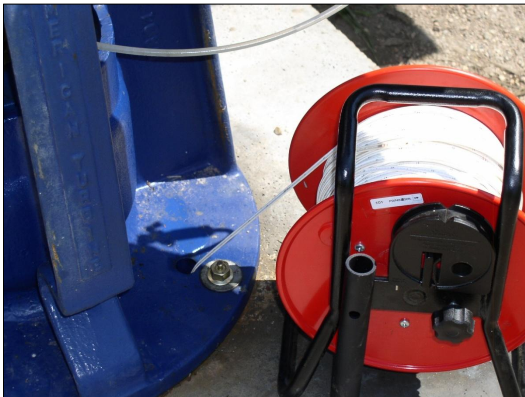
Figure 4.4 - Electric water level indicator.
