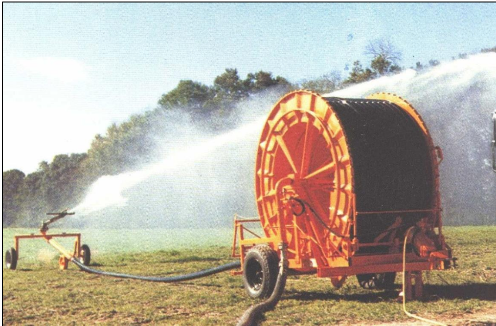
Figure B.4 - Traveling gun carriage and cart.
