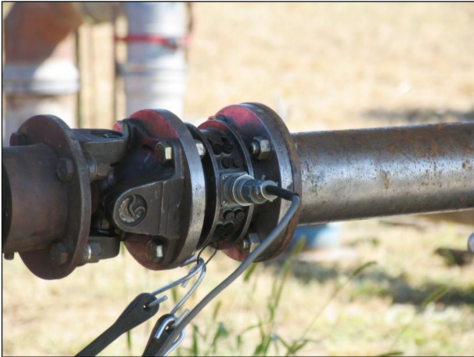
Figure 4.11 - Torque meter attached to engine drive shaft.
