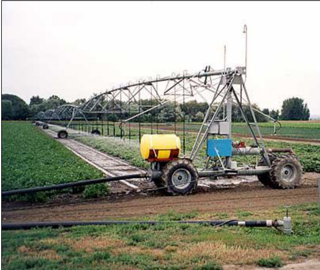
Figure B.3 - Linear move sprinkling system with drop nozzles.
