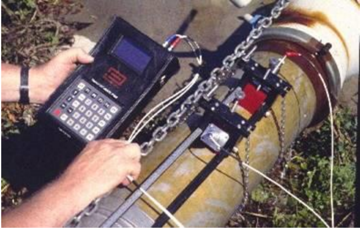
Figure 4.9 - Portable ultrasonic flow meter.
