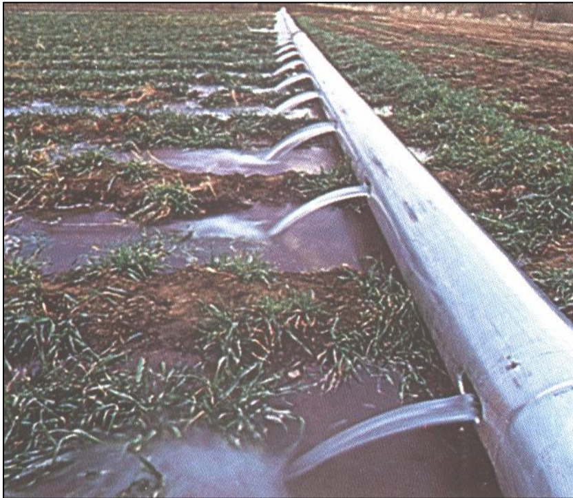
Figure B.1 - Gated pipe irrigating furrows.
